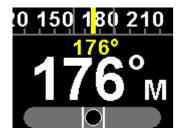
The F1 key pressed at a heading of 176 degrees. Currently the heading equals the course to steer as shown below the heading tape. No course steering indicators are shown.
