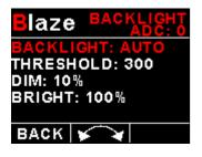
Allow 3 seconds for the display to adjust to the ambient lighting conditions when using the automatic backlight mode. The display will set the backlight to the dim setting if the ambient light is less then the threshold setting, alternatively the display will set the backlight to the bright setting if the ambient light is greater then the threshold setting. The ambient light received is shown as the ADC value in the top header. Use this value to set the threshold value.
