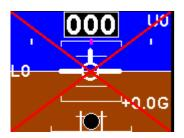
The display will have a red cross over the indicators to signal a SP-X sensor communication or sensor failure. Check the communication link between the AHRS-2 / MAG-2 and the SP-X sensors and that the SP-X sensors themselves are functional.
