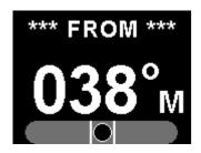
Press the F2 key to activate the reverse course display. This display remains active for about 5 seconds before reverting back to the normal heading display.
