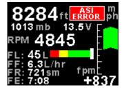
Airspeed sensor error. The instrument could have a faulty airspeed sensor in which case the instrument will then have to be returned to the factory. (Digital airspeed sensor models only)
