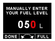
Press the F1 key during the main display screen to manually enter your current fuel level after fueling or defueling your aircraft. This function is only available if you have selected fuel level is calculated from fuel flow. Press the F2 key as a "quick fill button" to the full level.
