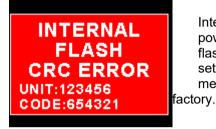
Internal flash CRC error. The instrument does a firmware check on the program when power is applied to the instrument. If the program is corrupt in any way then the internal flash CRC error will be displayed. Reload the instruments firmware and load default settings. If the error message still persists then it could possibly be an internal flash memory failure in which case the instrument will then have to be returned to the
