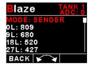
The fuel level sender needs to be calibrated before it can be used with this system. The calibration allows the system to learn the shape of your tank as well as any errors your fuel level sender or installation has.
