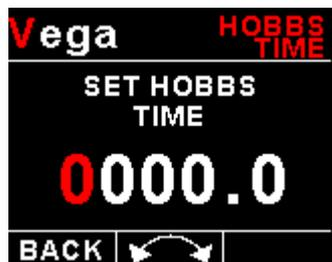
This function allows you to set the engine Hobbs meter to any value. Typically, you would use this function to set the Hobbs meter to the current known engine time. Use the rotary control to change the value. Press the rotary control to accept and exit the menu option. If the Hobbs code is set to another value beside zero, then the pilot will be prompted to enter the Hobbs access code before allowing him to change the Hobbs time. This feature is useful for chartered and flying school planes.
