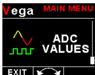
This menu displays the ADC values that have been read from the pressure and temperature sensor.
