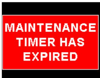
This function allows you to set an engine maintenance timer. This timer is set in engine hours and it will count down to zero when the engine RPM is greater than the "HOBBS RPM". A good use for this function is to set the hours until your next spark plug change or engine inspection. Use the rotary control to change the value.
