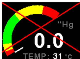
The red cross over the display means the MAP-3 has lost communications with the external RDAC unit. Check the wiring between the MAP-3 instrument and the RDAC unit. This error message is only available when the external RDAC is selected as the data source.
