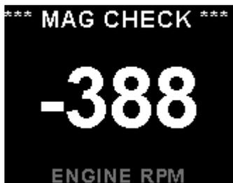
Press the F2/Down button once you have reached your normal run-up RPM. The display will show the RPM deviation from when the magneto function was activated. Any RPM drops will be displayed as a negative RPM value, a positive reading indicates an increase in RPM.
