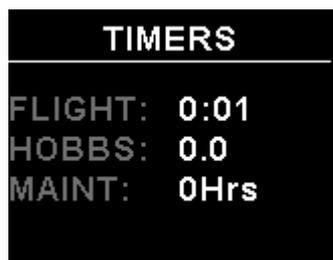
This display can be accessed by rotating the rotary control during the normal display mode. The flight, Hobbs and Maintenance Timers are shown.
