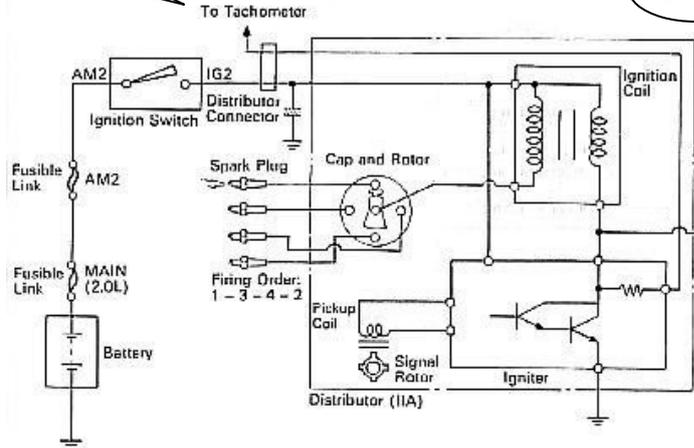
Connect rev counter input of MAP-3 to this line (Insert 10k resistor in series). Ensure you have a connection from the MAP-3 ground to the engine block.
