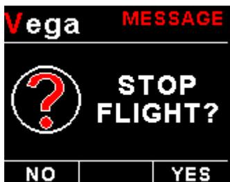
Press the F1/Up button during the normal display mode to manually start/stop a flight. This key is only active if the MAP-3 is setup to select the manual flight option under the "TIMERS" setup menu.
