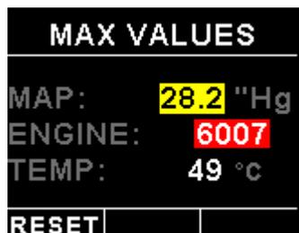
This display can be accessed by rotating the rotary control during the normal display mode. Press the F1/Up button when the max values display is showing to reset the maximum values to the current values.
