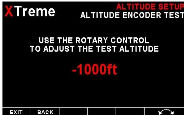
The XTreme-EFIS has a built in altitude encoder test function to test the installation between the XTreme-EFIS and CNV-ALT to the transponder.
