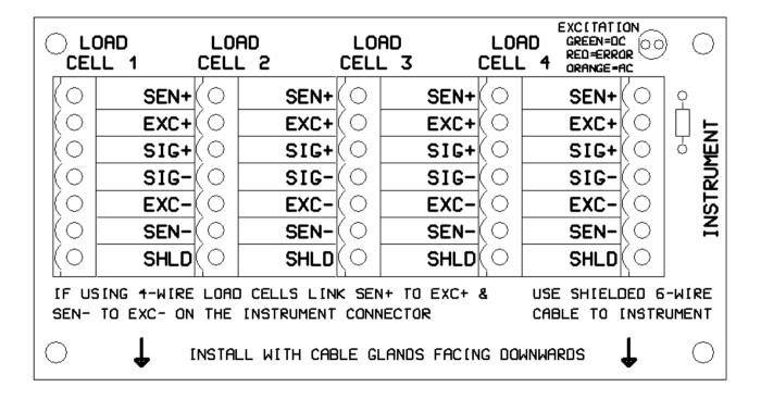
Note: Install with cable glands facing downwards and with cable drip loops
