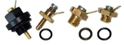
These plugs are available in different thread sizes to suit coolant plugs or bleed screws originally fitted to engines. 1/2BSP, M6x1, M10x1, M12x14tpi, others
