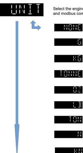
Select the engineering display units. The display units are used for the ASCII out printing and modbus communications.
