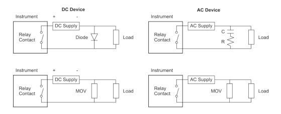
An optional noise suppression device can be ordered. Install these devices as close to the load as possible.
