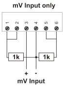
Link Exc+ to Sense+ and link Exc- to Sense-Set Signal - to midpoint using 2x 1k +-1% resistors
