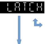
The alarm can be set to remain activated even if the alarm condition has gone. When the alarm condition has gone then the alarm latch can be reset by either a digital input or via the front push buttons.
