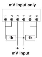
Link Exc+ to Sense+ and link Exc- to Sense-Set Signal - to midpoint using 2x 1k +-1% resistors
