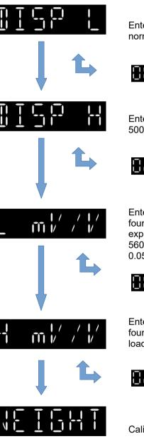
Enter the value in engineering units of the low calibration point of the system. This is normally zero.
