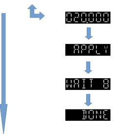
Use the front panel push buttons to enter the display value that corresponds to the high calibration weight.
